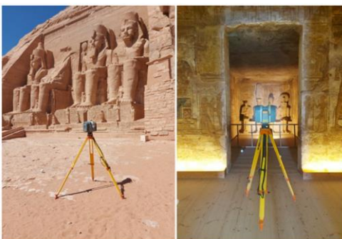
Figure 4. Surveying Abu Simbel Temple's interior and exterior parts with terrestrial laser scanner TX6.
