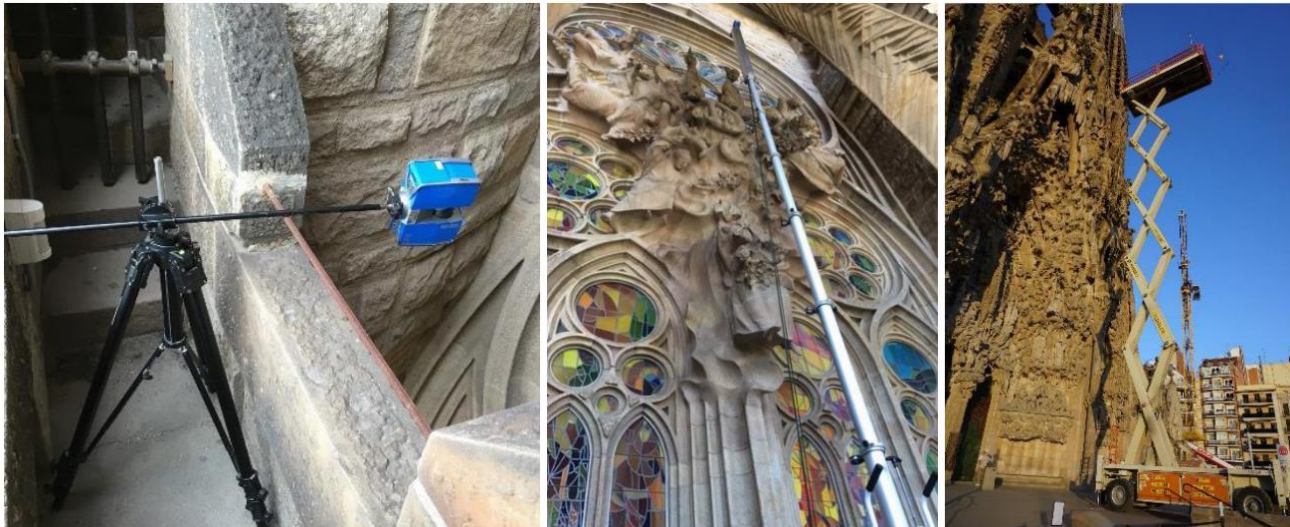
Figure 26 Scanning methods of Sagrada Familia [15]
