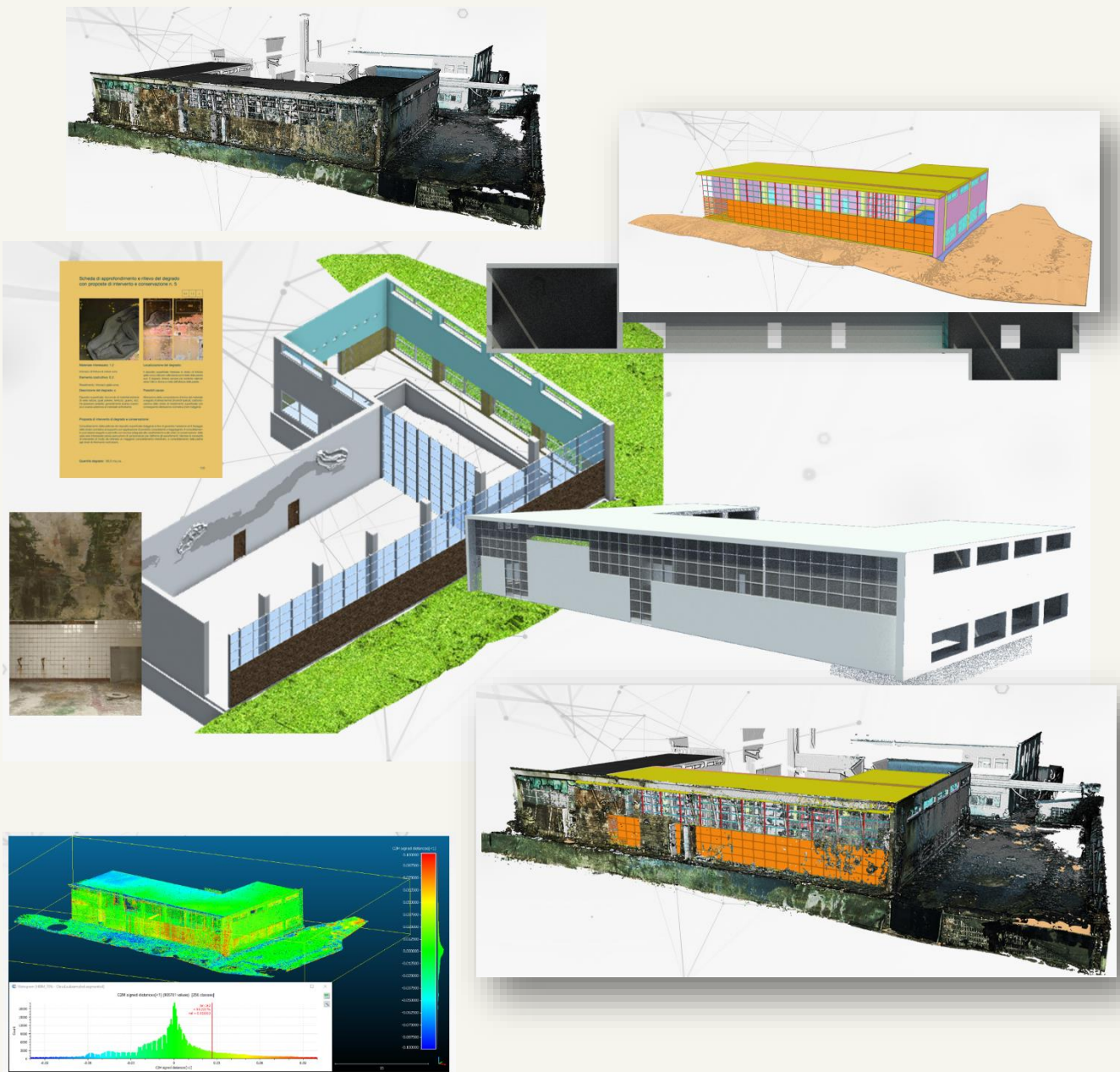
Figure 31 from laserscan survey to HBIM model and analysis
